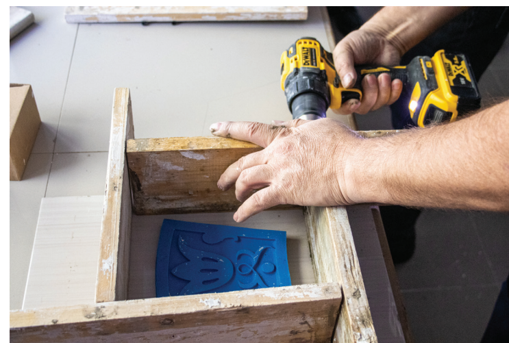
Ornamental piece / The Turkish Bath in Iași, silicon and gypsum negatives casting process, dimension variable, 2020-2024
